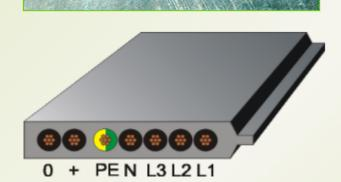
The connecting devices are contacted by piercing contacts to the TC-ER cable power bus.
